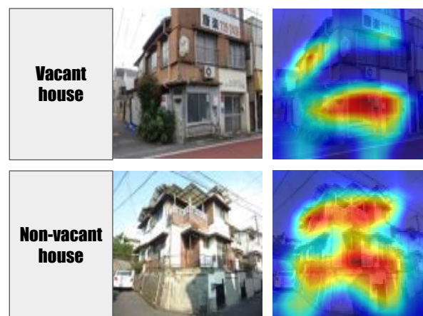
Fig 9 Grad-CAM attention in building opening parts
