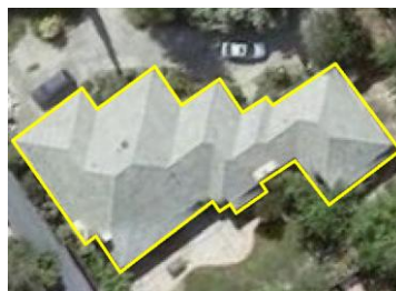
Figure 2: Building polygon on satellite image, expressed as RRLRLRLRLRRRLRLRLRLR
