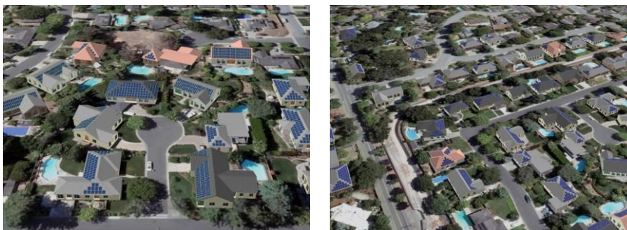
Figure 8: Automatically generated 3D urban model by polygon rectification
