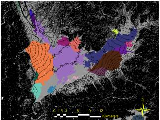
Figure 4. Alluvial fans found by the algorithm in Kofu Basin area. Each fans originated from different apices are colored differently.
