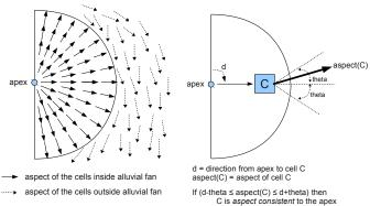
Figure 2. Aspect distribution of alluvial Figure 3. Aspect Consistency Test fan
