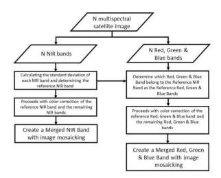
Figure 1. Color correction algorithm flowchart
