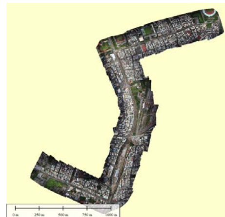
Figure 4. An orthophoto result for post-disaster assessment
