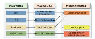
Figure 1. Wi-Fi AP information gathering procedure utilizing MMS
